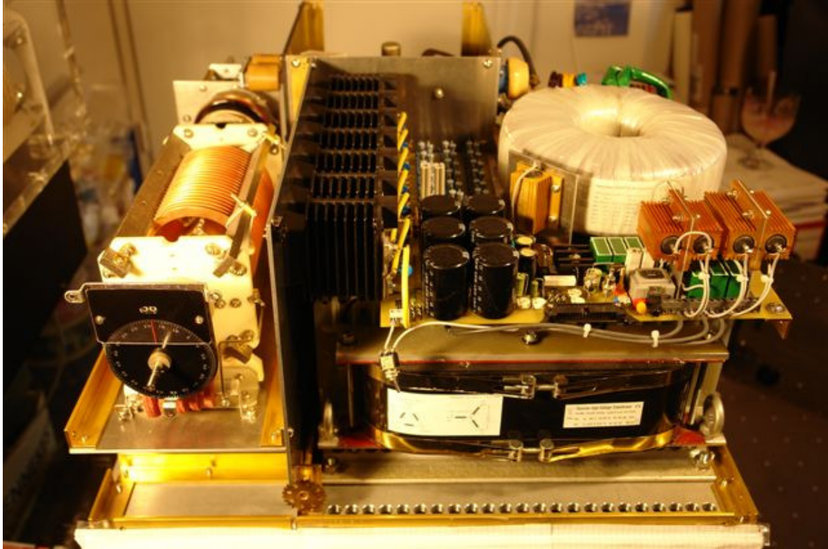
Fig. 5: Front view without front panel, side plates and back board. Three-phase alternating current high voltage plate transformer (bottom right), central power supply board with toroidal transformer (above plate transformer), 7 x Zener diodes for the screen grid (center top), roller inductor (top left), cogwheel (bottom center) for switching the control grid transformer parts (compensating the input capacitance of the tube and neutralizing the tube itself, 11 switching positions for all amateur short wave bands)
