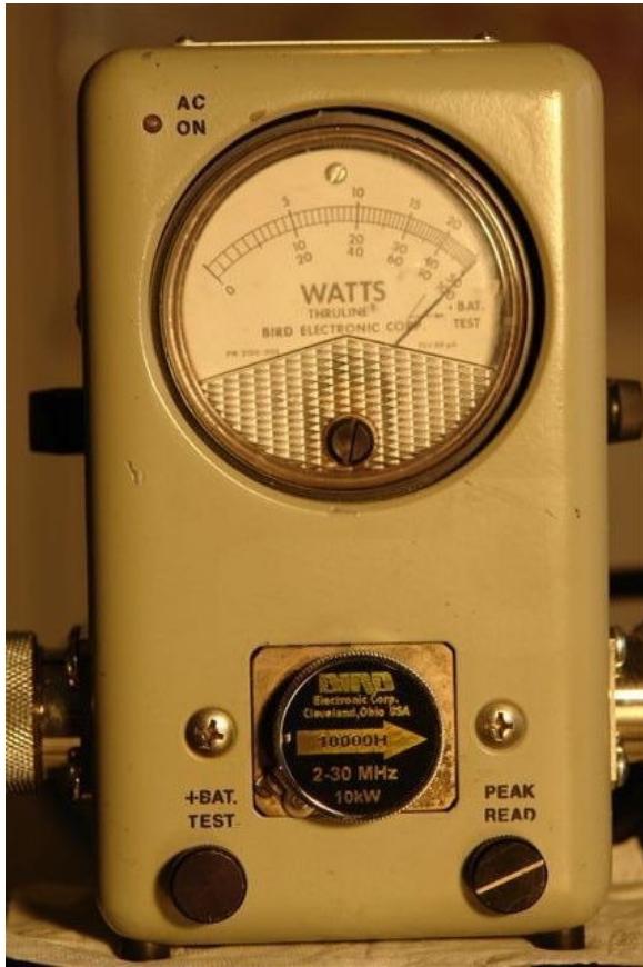
Fig.16: Proof of output power: With an input of only 70 W on 40 m the Tsunami power amplifier provides an output of 10.1 KW.
