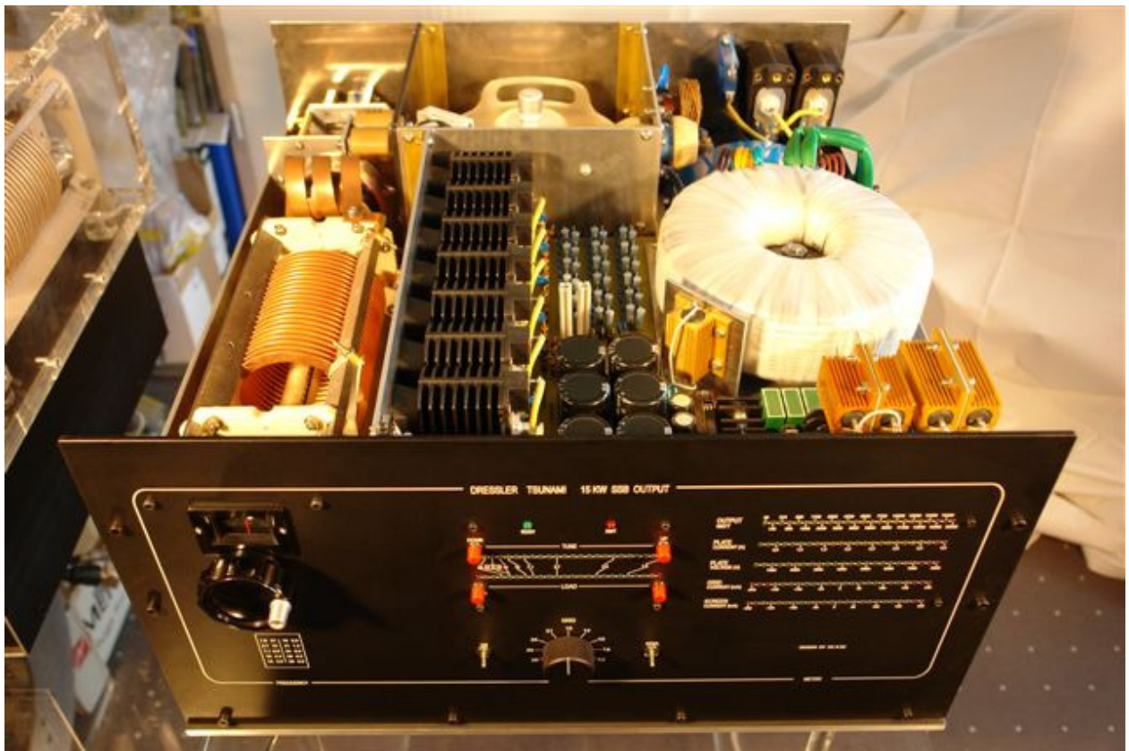
Fig. 14: Finished Tsunami power amplifier: Does anybody know of a smaller 15 KW SSB output stage?
